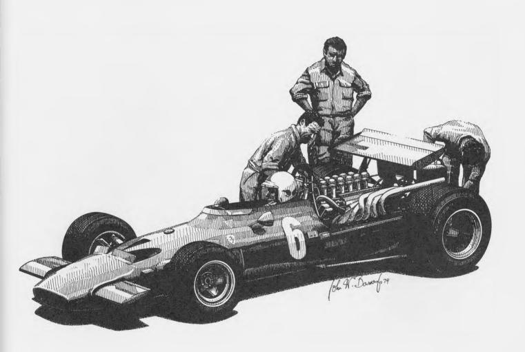
Since the introduction of the rear wing on Grand Prix cars in 1968, the full potential of aerodynamics in racing was very quickly realized. If a wing would provide better traction and stability, why not utilize the whole body as a primary aerodynamic component to do the same thing? This Lotus did, in its beautiful wedge-shaped 498 cars of 1969. The bodies of all future Formula I cars would have to follow strict aerodynamic laws.
